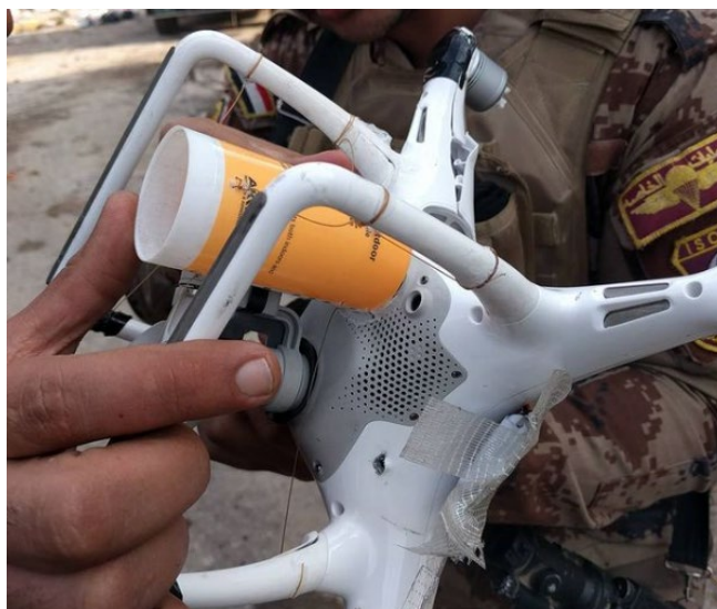
Captured ISIS' COT sUAV modified to carry grenade-sized explosive payload xviii
